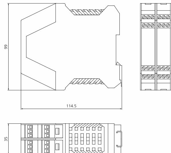
**Abmessungen SR-0 in mm:**
