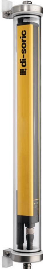
Watertight protective housings allow light curtains and light grids to be used in a harsh working environments with exposure to water and steam. Thanks to its inert components, no residuals or contamination are left when the light curtains/grids are washed down or when they come directly in contact with food. This makes **WTF** and **WTHF** protective housings suitable for the Food & Beverage industry.
