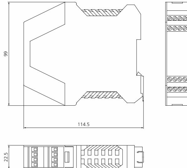
**Abmessungen SR-M in mm:**
